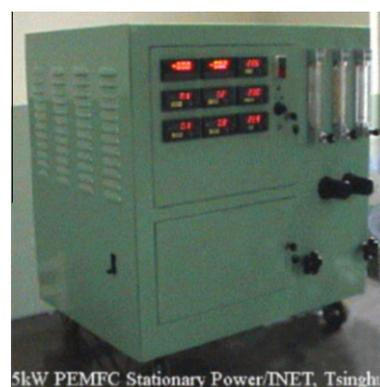
**Fig. 13.** A 5 kW PEM fuel cell stationary power [63].
