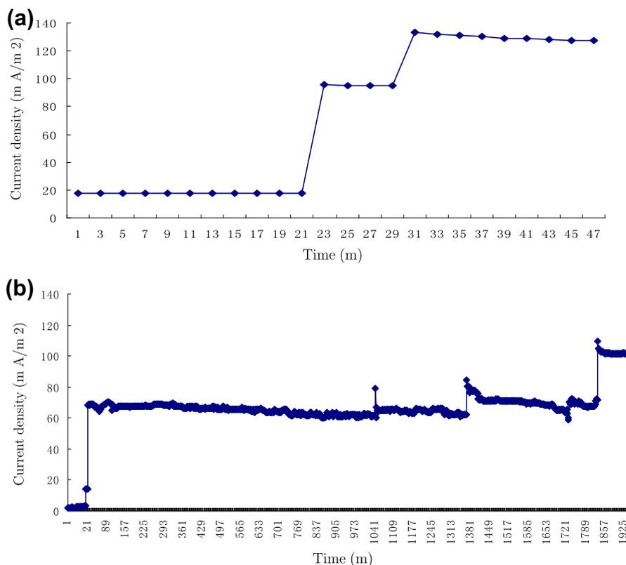
**Fig. 4.** Current generation in MFC after replacing the existing catholyte (a) and anolyte (b) with fresh medium to remove suspended bacterial biomass. The current is measured using  $1000\ \Omega$  external resistance.
