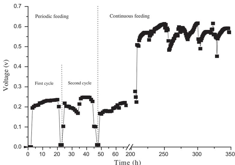
Fig. 2. Voltage generated using membrane-less MFC using different organic nutrient feeding operations (periodic and continuous nutrient loading).
