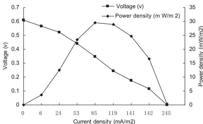
Fig. 3. Polarization and power density curves of MFC.
